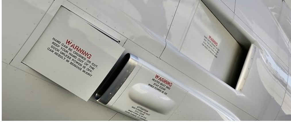
Figure 4.2: Environmental control system inlets Boeing 787-9, reproduced from [11]
