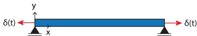
Fig. 8 Schematic of the geometry and boundary conditions for the bar spall benchmark. The axial displacement signal \delta(t) in Equation (36) is applied at the two ends of the bar, while two roller supports restrain the transverse displacement
