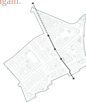
The main distribution pipe of a regional district heating network runs along an important axis of Moerwijk. Some parts are dug in, and some are placed with directed drilling, needing no excavation.
