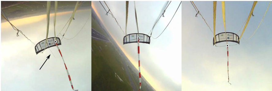
Fig. 15.4 Wing and bridle line system during a downloop figure eight maneuver performing a right turn (left) and following straight flight diagonally upwards (center) and during retraction of the kite (right). Video stills taken from the kite control unit (24 November 2010)
