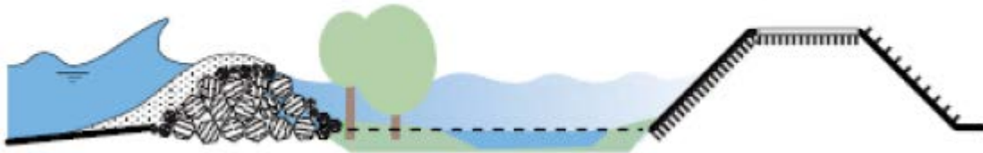
Figure 64. Concept design of nature enhancing flood defence. Source: (van Berchum et al., 2015)
