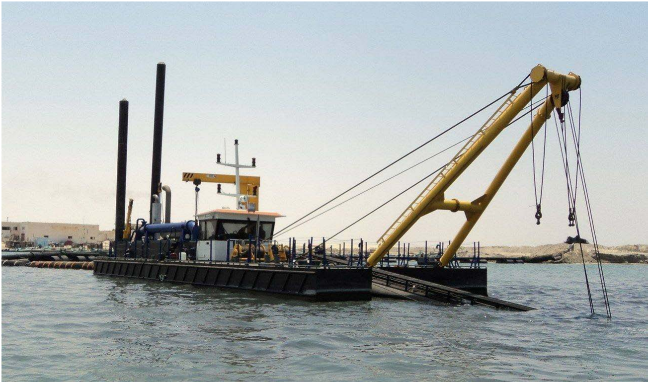
Figure 55. CSD650-18 cutter suction dredger. Source: (Damen, 2109)
