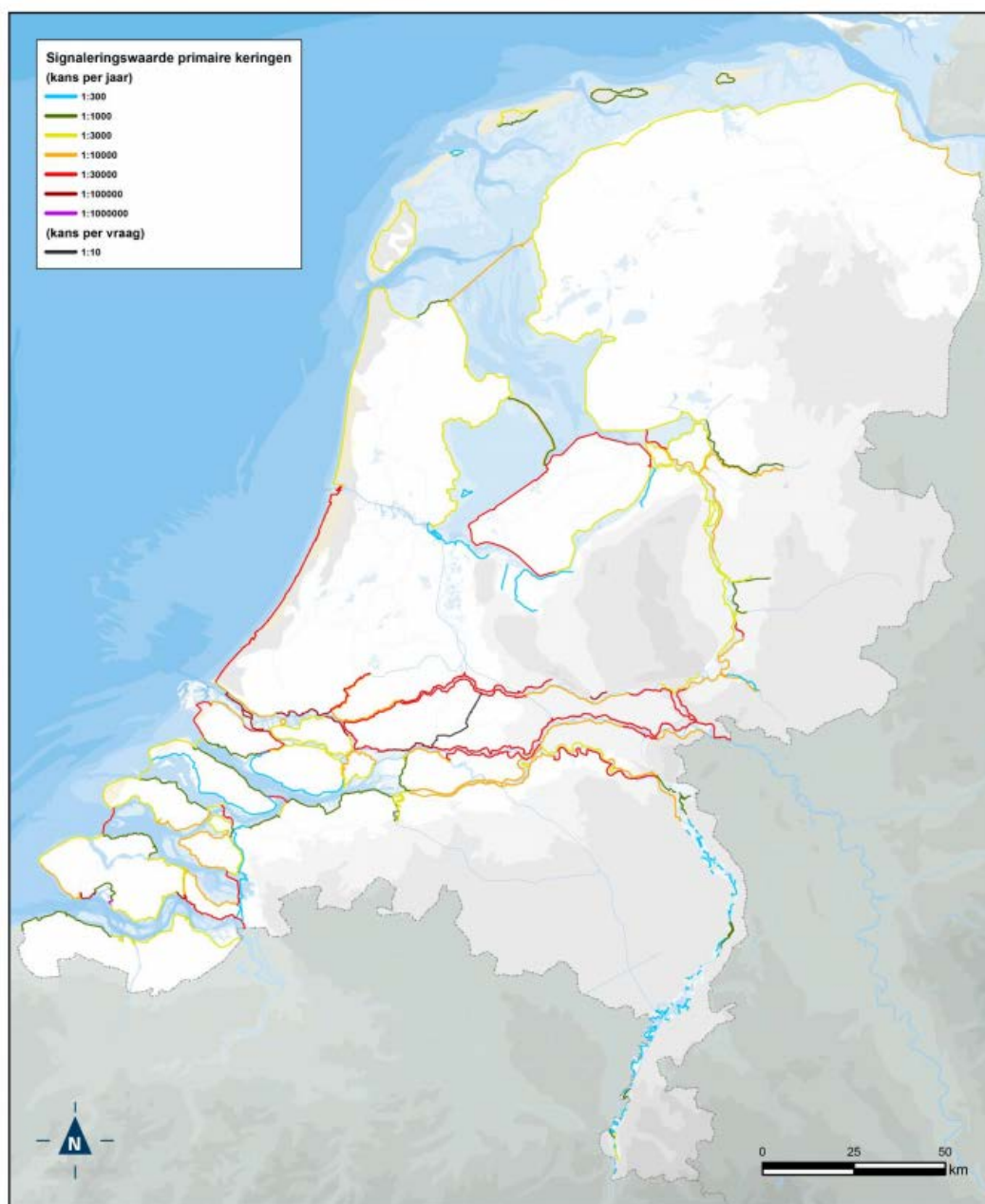
Figure 18. Flood safety standard in The Netherlands, based on failure probabilities per dike sections. Source: (Ministerie van Infrastructuur en Milieu., 2016)
