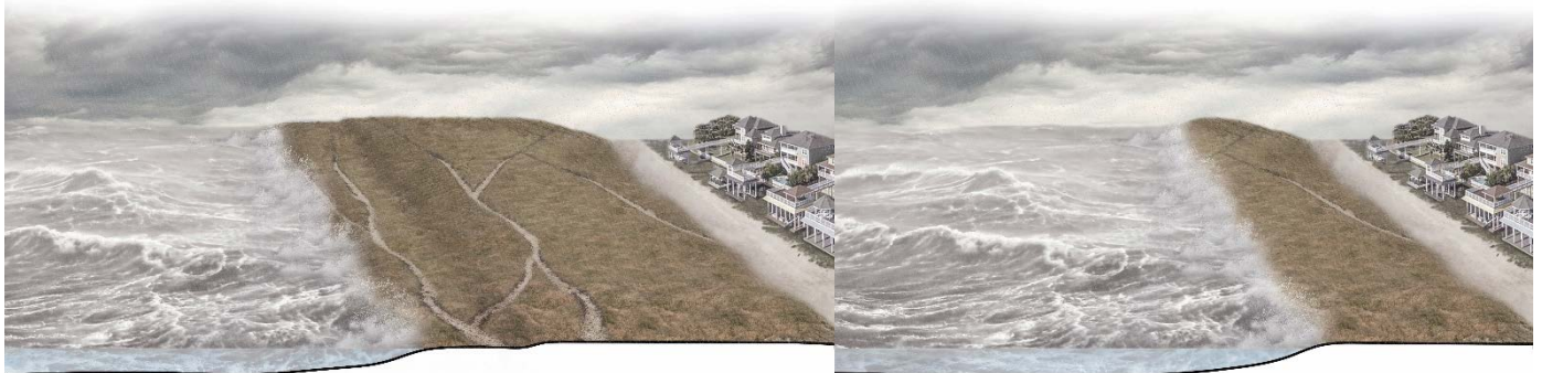
Figure 24. Illustration of the traditional flood protection dune at the beginning (left) and during the storm (right).
