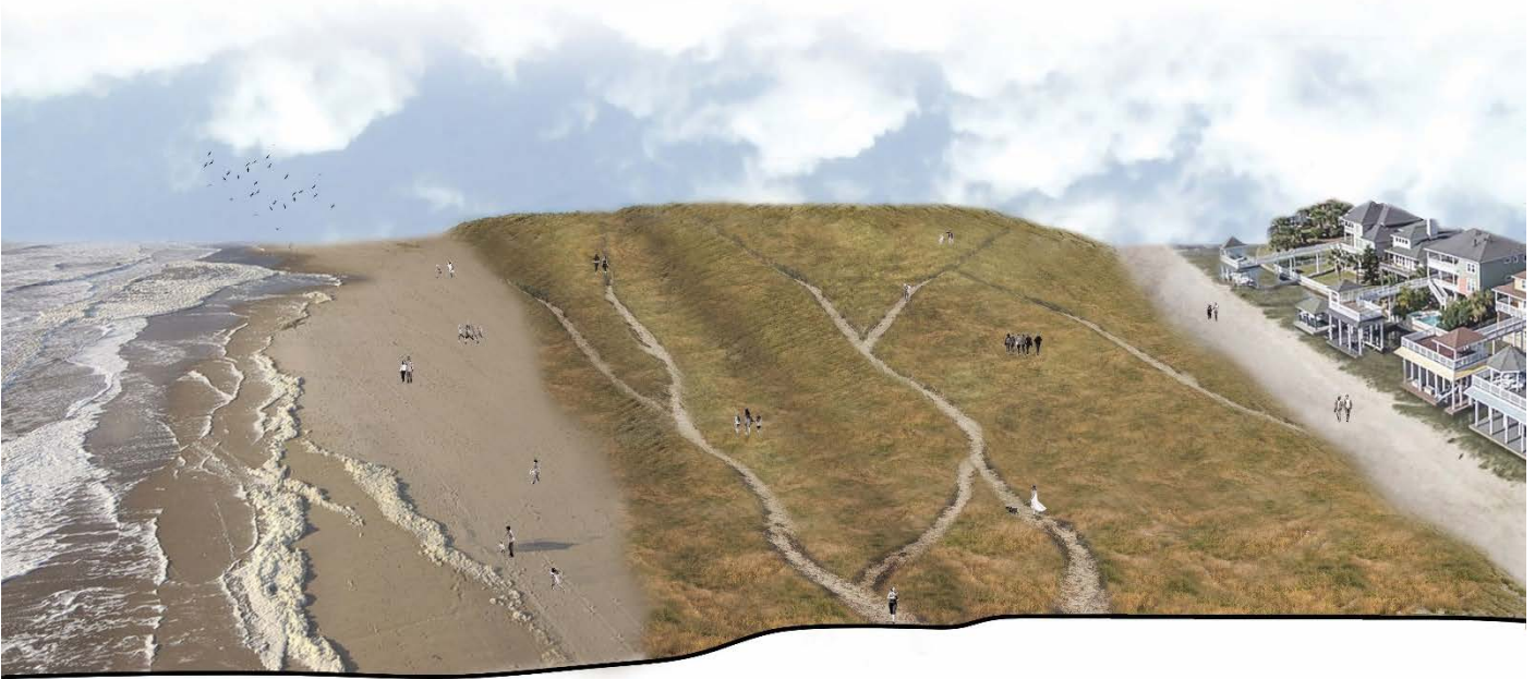
Figure 23. Illustration of the traditional flood protection dune concept design.
