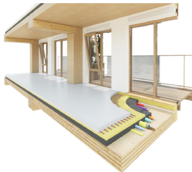
Figure: Section detail of the storey showing floor layers.
