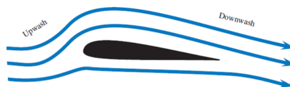
Figure 7.6: Upwash effect of an airfoil. 3
