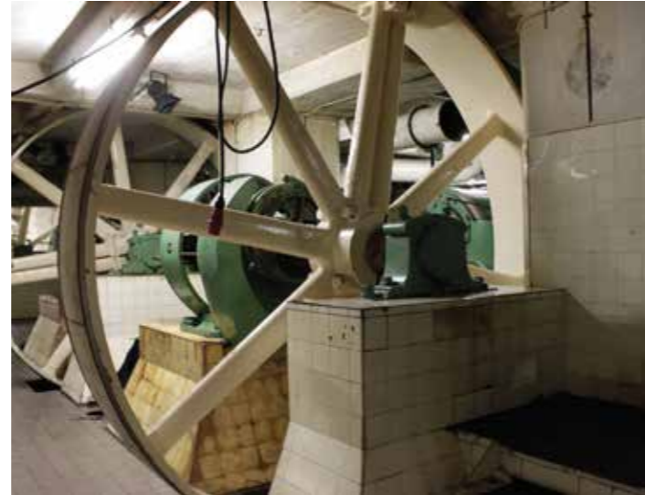
Electro-motors with flywheels which power the pneumatic pumps they were cooled by cooling pumps which used water of the Maashaven. These motors really give meaning to the basement as to what it function was.
