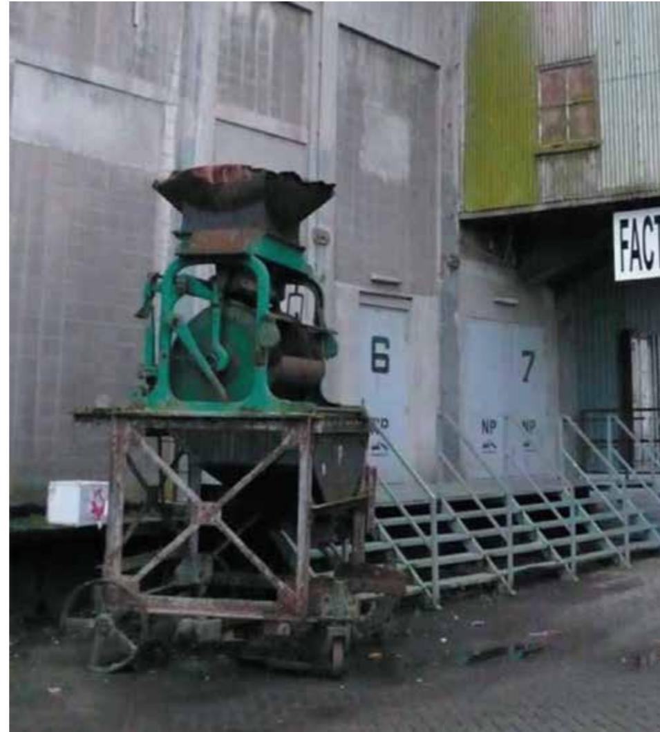
Moveable scale to weigh the grain (Source: Transformers (2008), Cultural Value report)
