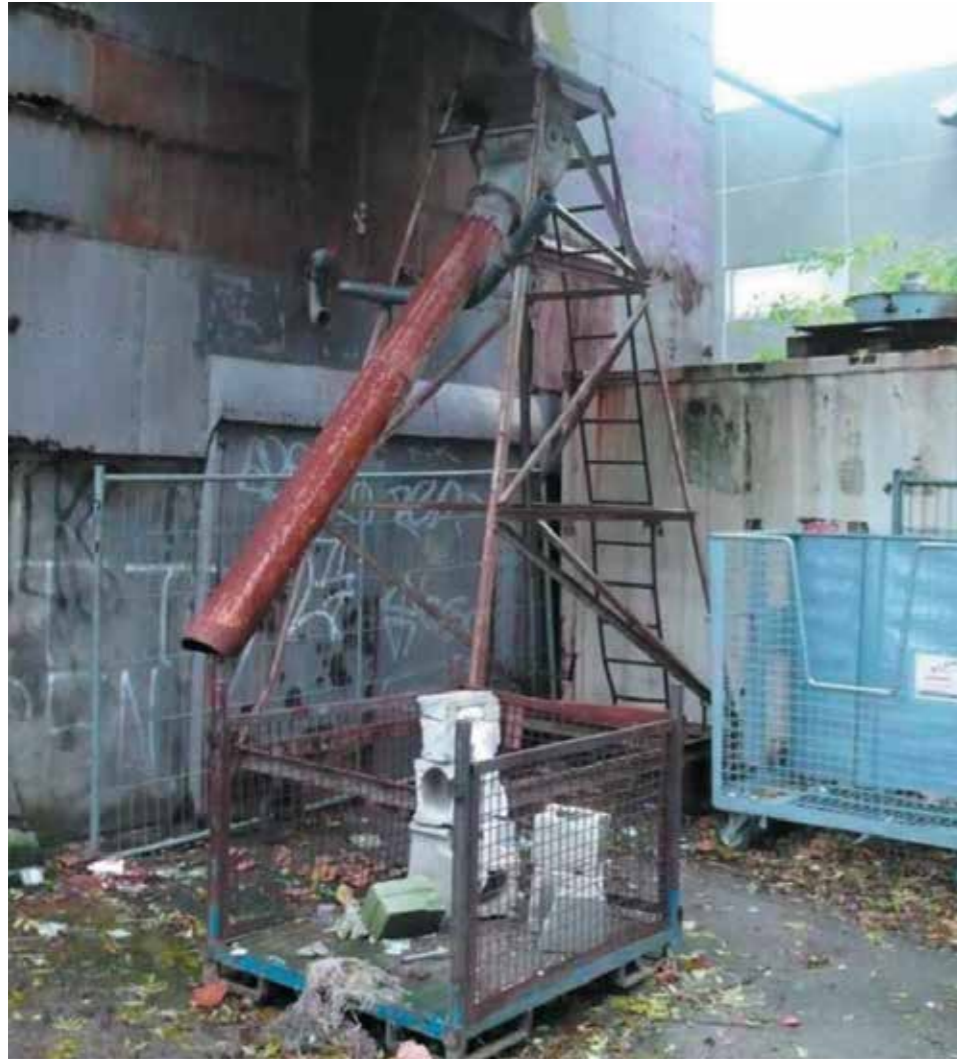
Moveable telescope tube to collect grain from the silos (Source: Transformers (2008), Cultural Value report)
