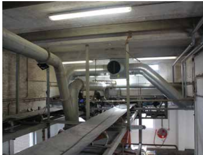
Conveyer belts which transport the grain from the Cup elevators to the distribution pipes for the silo's
