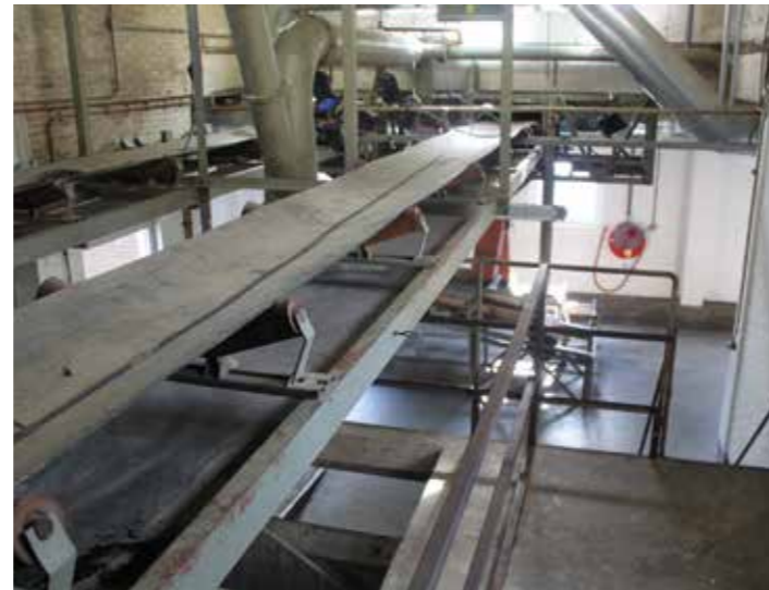
Conveyer belts which transport the grain from the Cup elevators to the distribution pipes for the silo's
