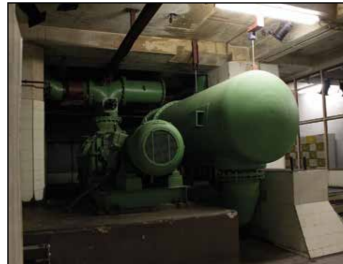
Pneumatic pumps which create a vaccum (suction) which make it possible for the elevators and cranes outside to suck 400 tons of grain out of the boats per hour and transport them indoor. the machines were made by SIEMENS
