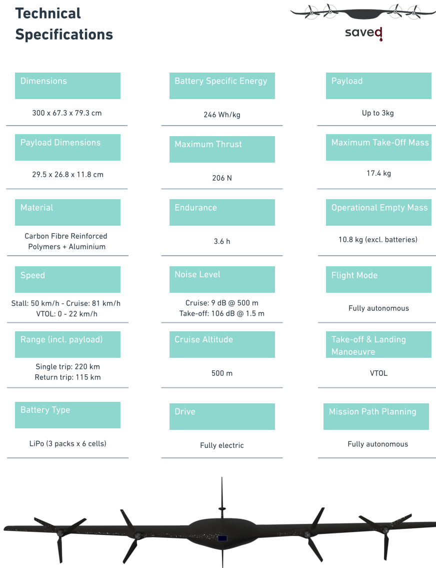
Figure 19.1: SAVED's technical specifications.
