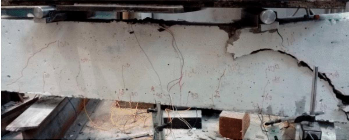
Figure 5.4: Experimental failure crack pattern of benchmark beam CB1
