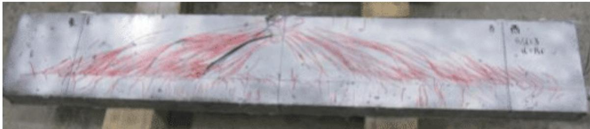
(a) Experimental failure crack pattern
