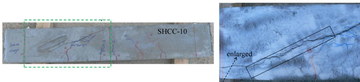
**Figure 5.47:** Experimental failure crack pattern of benchmark beam H10Q2
