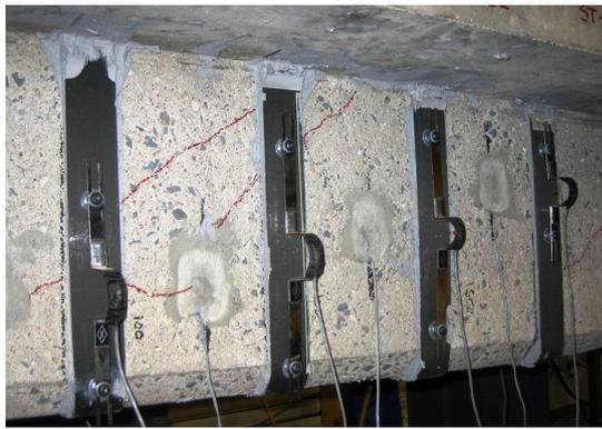
(a) L-shaped steel strips for shear strengthening of concrete beams [42]
