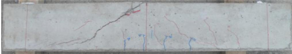
Figure 5.10: Experimental failure crack pattern of benchmark beam CB2
