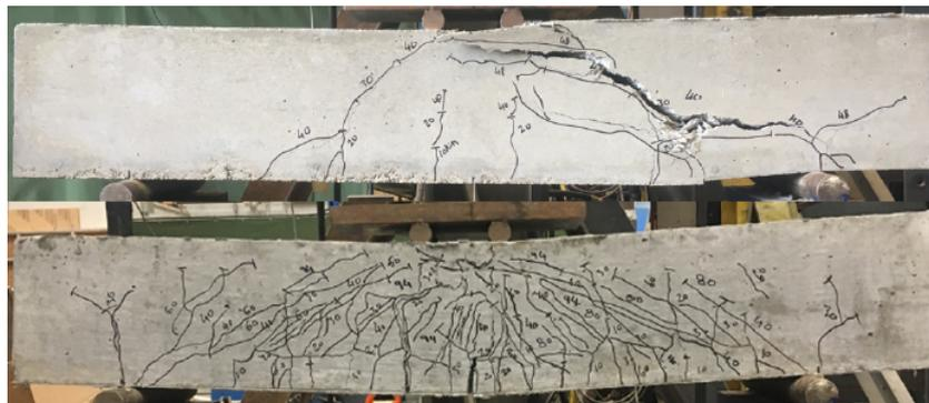
(b) Failure cracking pattern of the test beam with of normal concrete (above), and SHCC-PVA8 beam (below)
