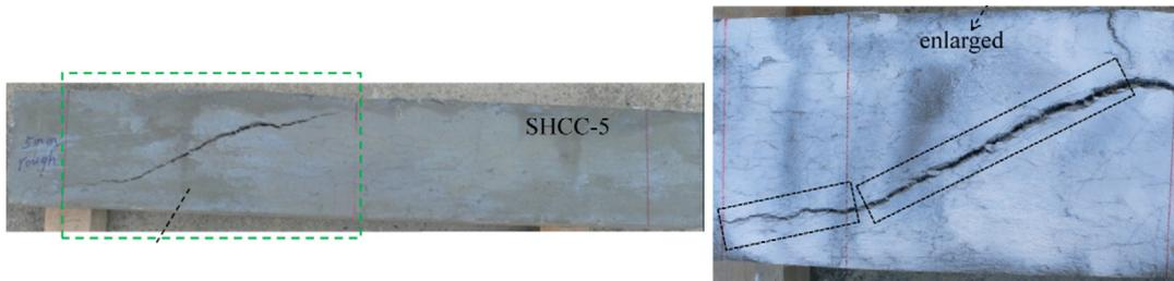
Figure 5.43: Experimental failure crack pattern of benchmark beam H5Q2
