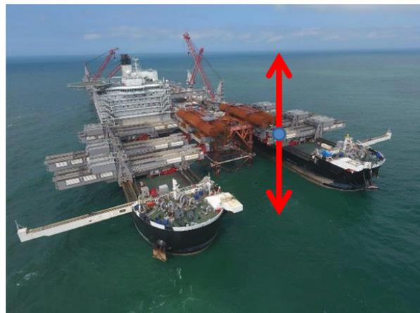
Figure 1: Heave motion at the location of topside lift system
