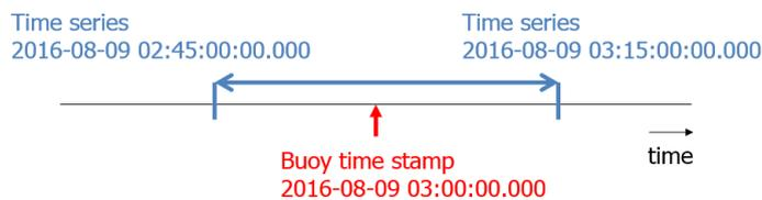
Figure 6.15: Selection of the time interval. The buoy has a time stamp every half hour, the time series is selected a quarter of an hour before and after the buoy time stamp
