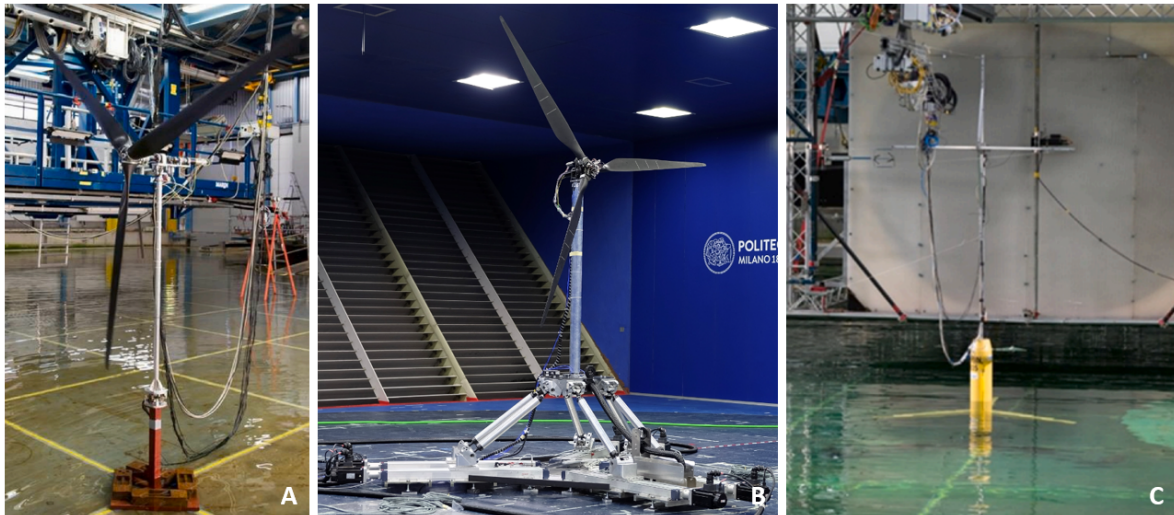
Figure 3.1: Examples of model testing. A: A turbine with modified airfoils on a fixed support [42], B: A turbine on top of a hexapod to simulate hydrodynamic forces [44], C: A floater with winches to simulate aerodynamic forces [42]
