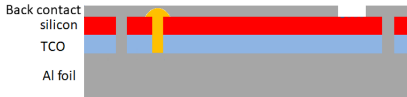
Figure 5.31: Cross-sectional view of the cell after removing the lift-off ink [24]
