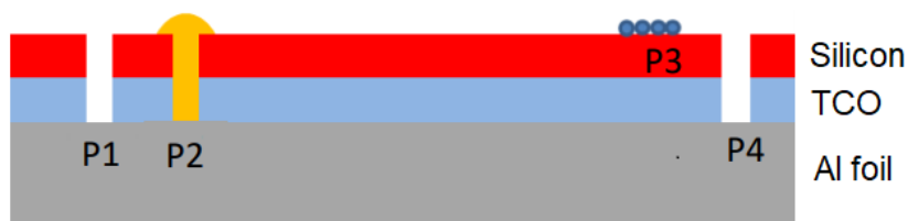
Figure 5.29: Cross-sectional view of laser scribes P1,P2, P3, TCO fill ink at P2 ink and lift-off ink at P3 [24]
