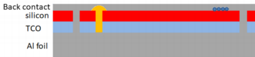
Figure 5.30: Cross-sectional view of back contact deposited on top of the scribes [24]
