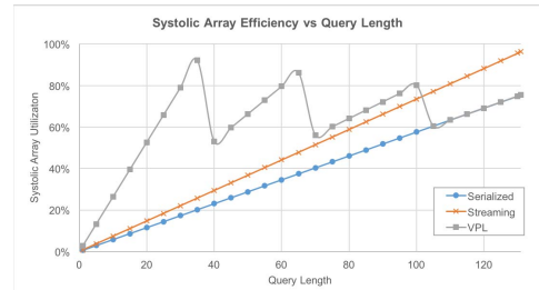
Figure 5. Systolic array efficiency dependence on query length (data set: 100 alignments with variable query length and target length 400).
