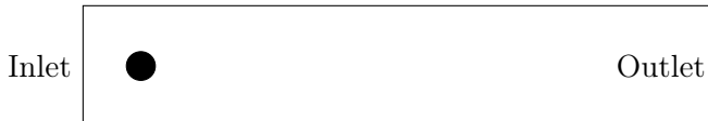
Figure 7.14.: Schematic of the domain for the flow around a cylinder test case
