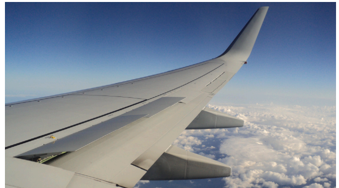
(b) A Boeing B737-800 using spoilers to control the rate of descent.
