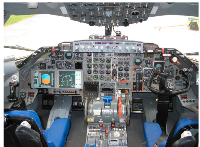
Fig. 5. ATTAS cockpit view, with experiment pilot seat on the left and safety pilot seat on the right.
