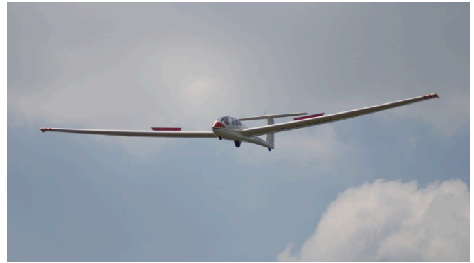
(a) A glider using spoilers to directly manipulate drag and control the flight path angle during final approach.
