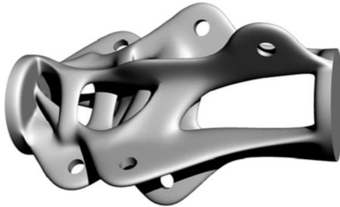
Figure 1.1: An example of a structure generated using topology optimization that seems difficult-to-clean, from Galjaard et al., 2015.
