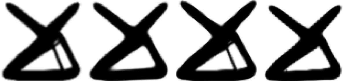
(a) The final design of the iron setup using the SIMP method. The objective value is 68.55.
