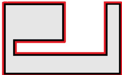
(d) The shell is fully converged and has become one with the rest of the structure. This design has most likely the best objective value, but it is no longer cleanable.
