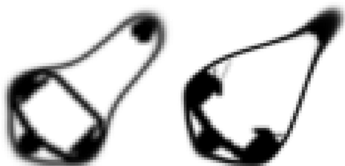
(a) The four points setup with  $r_\phi = 16$  and  $\eta_1 = 0.15$ . The limited convexity of the shell is seen at the top right and bottom left. The objective value is 21.92.
