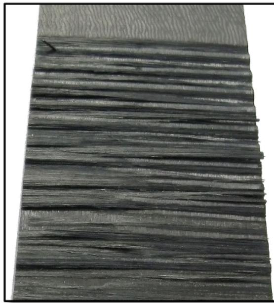
Figure 2.7: Fibre bridging of an 90^\circ//90^\circ interface [54]
