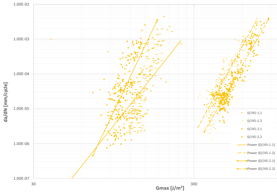
Figure C.1: da/dN vs G_{max} graph of the 0^\circ//45^\circ interface.
