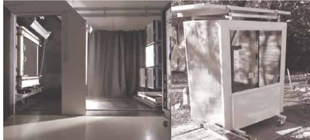
Fig. 13 Left: Indoor calorimeter, Fraunhofer ISE, right: Test chamber, Valencia, Spain.
