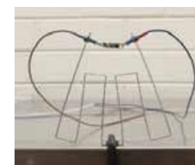
Figure 3: Example of using a waved-shape layout for the bottom layer of the thin-walled module
