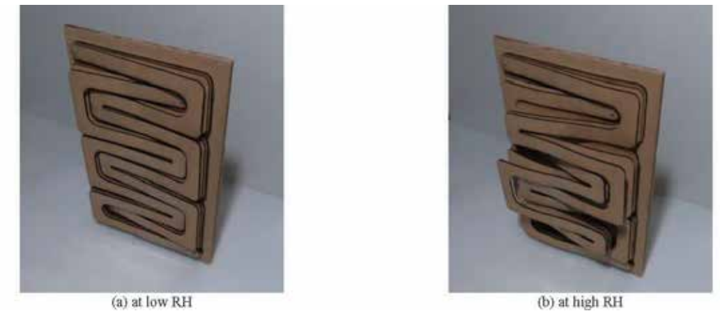
Fig. 4 Morphing process of the prototype for a basic module for the modular wall/partition system (low RH = 33%, high RH = 85%)
