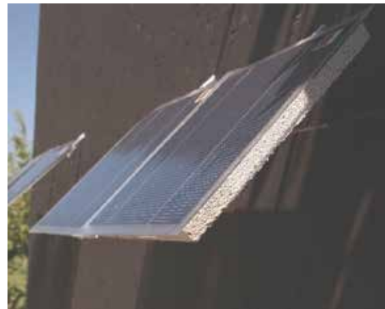
Fig. 1 The bionic leaf, consisting of a photovoltaic cell (top), a evaporative matrix (bottom) and a supporting stem for water transport.
