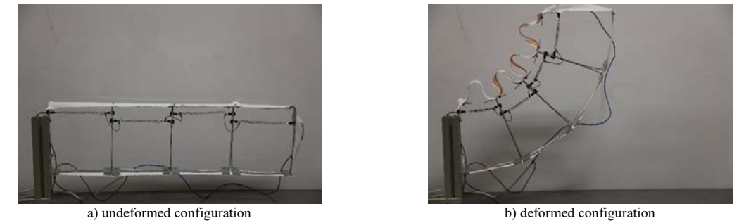
Figure 5: Four-module morphing system with a thin strip of shading fabric
