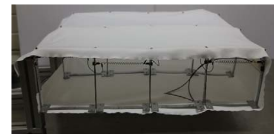
Figure 8: Shading prototype after recovery of the initial undeformed configuration (i.e. after the morphing depicted in Figure 7)
