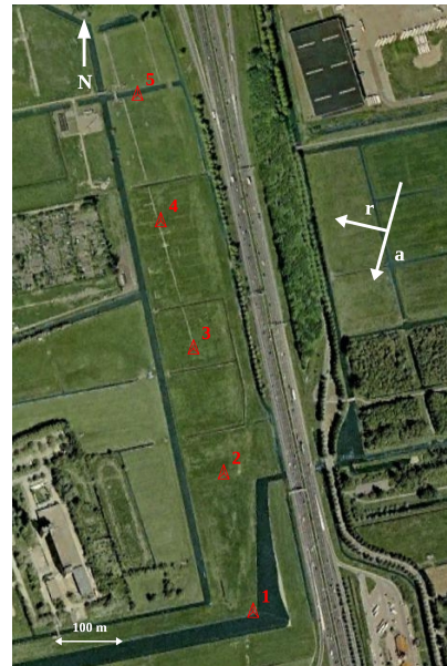
Fig. 9. Delft CR experiment setup for ENVISAT ASAR descending acquisitions. CR and their numbers are marked in red as shown in the GoogleEarth (optical image date: May 19, 2004) [21].
