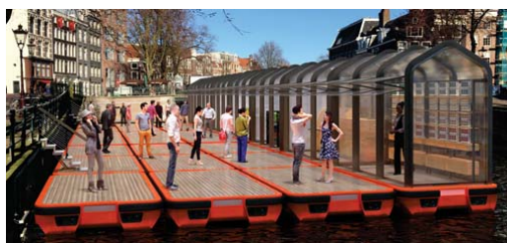
Figure 2.3: Roboat's concept of creating floating structures from square modules Wang et al. [51].
