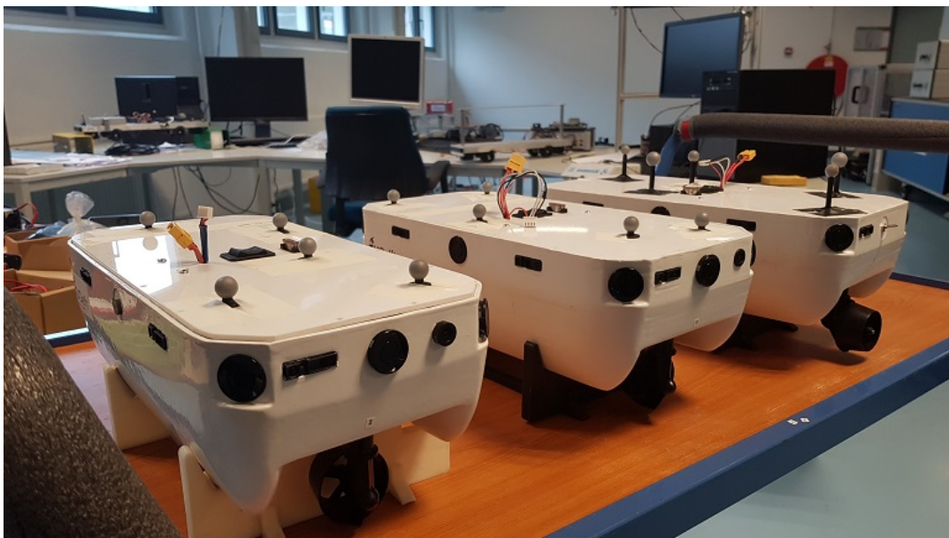
Figure 5.1: Delfia-* vessels, that will act as modules of the fleet system, to perform automated assembly and control.
