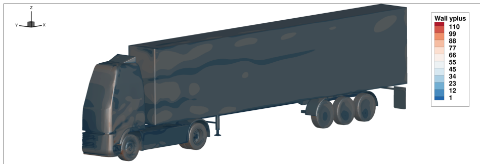
Figure 4.1: y^+ contour over truck
