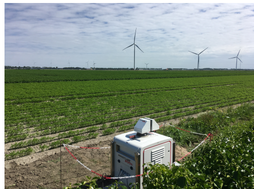
Figure 5.2: Leosphere Vaisala Windcube 200S Scanning LiDAR placed in the TIADE test site in Wieringermeer, The Netherlands
