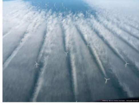
(b) Partial-wake conditions seen in the photo taken from Horns Rev 2 wind farm (figure taken from [5])
