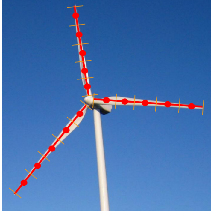
Figure 4.1: Representation of the actuator line method for a wind turbine rotor
