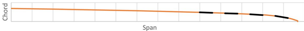
Figure 5.5: Gurney flaps (Blue thick line) shown on wind turbine blade (only a part of the blade is shown)
