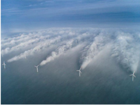
(a) Full-wake conditions seen in the photo taken from Horns Rev wind farm (Courtesy: Vattenfall. Photographer is Christian Steiness)
