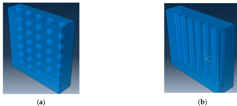
Figure 12. FE models with different form of macro capsules; (a) spheres and (b) pipes.
