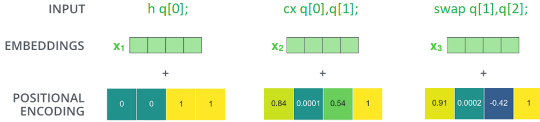
Figure 2: Graphical example of positional encoding. A positional encoding vector is added to each word embedding vector. The values of the positional encoding vector depend on the position of the input in the sequence. Adapted from [30]
