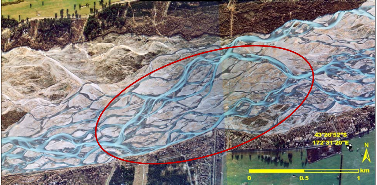
Figure 1. Braided reach of the Waimakariri River near Cross-Bank. Typical compound bar is highlighted by red circle. Flow is from left to right.
