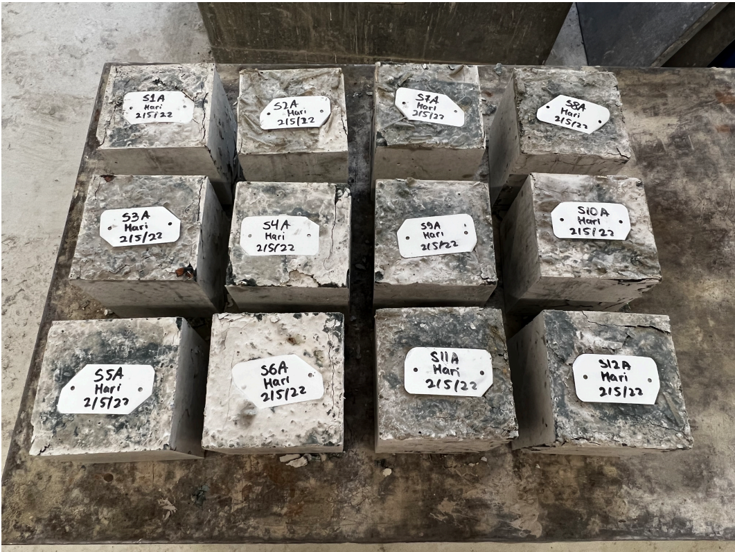
Figure 4.4: Part of Phase 2 samples after compression tests.
