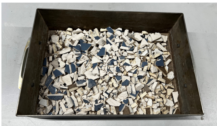
Figure 3.5: Ceramic tiles, 8 to 16mm in size, after crushing and sieving
