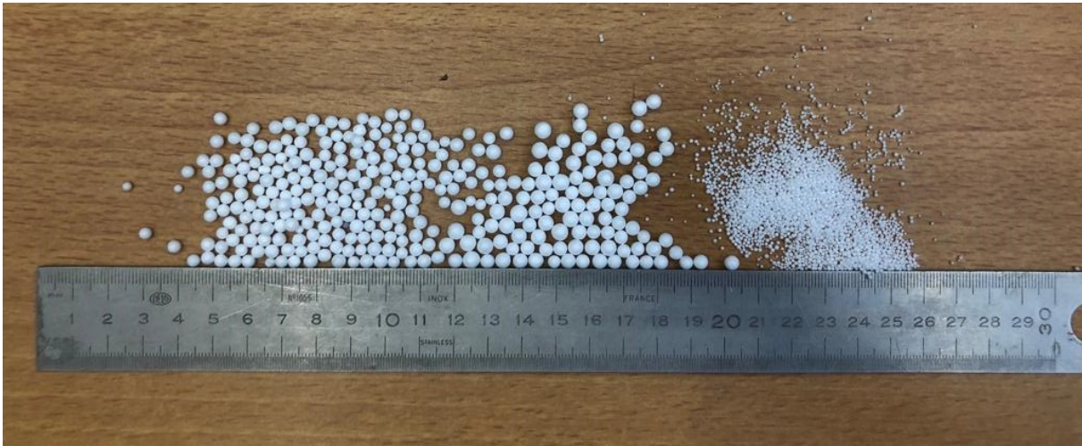
Figure 3.15: Individual foam particles used to simulate air voids in this research
