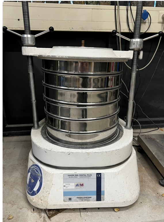
(b) Vibrating tray sieve used for particle separation
