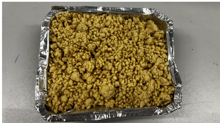
Figure 3.8: Mineral fibers used in the project
