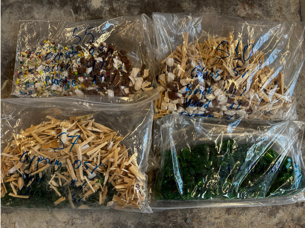
Figure 3.18: Contaminants are kept separately from the aggregates prior to mixing (part of Step 1)
