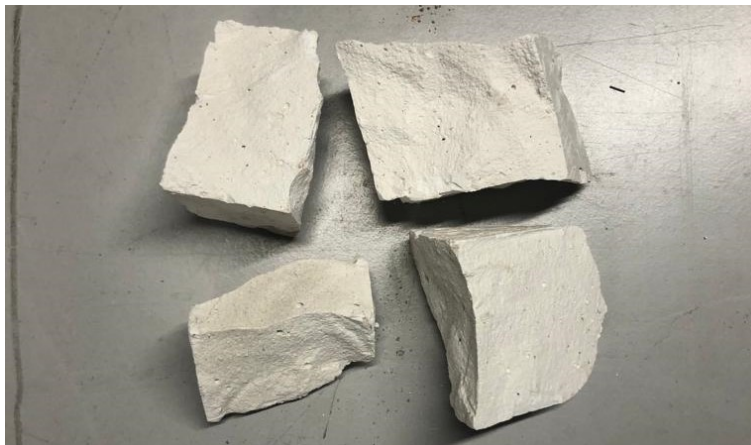
Figure 3.4: Raw gypsum blocks ready for crushing and sieving
