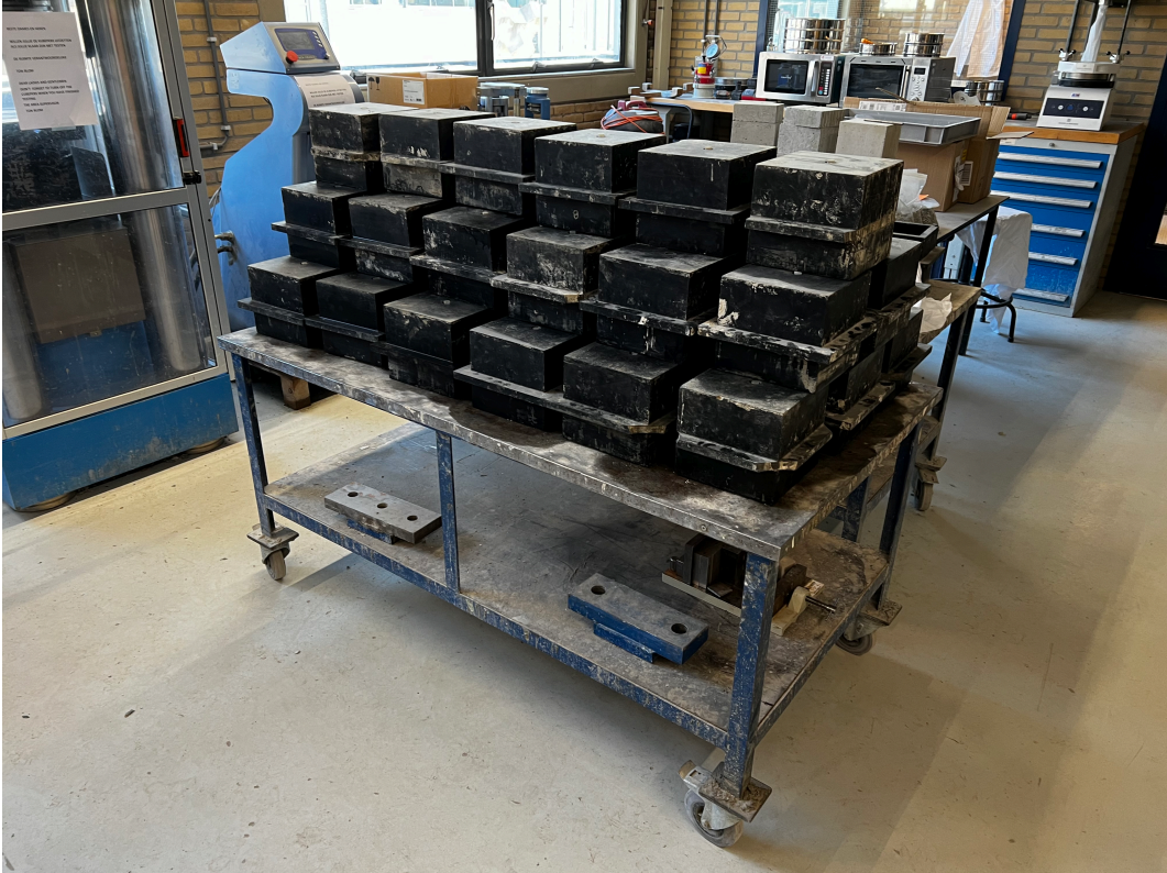
Figure 3.19: Oiled moulds are left upside down to unload all excess oil (part of Step 2)
