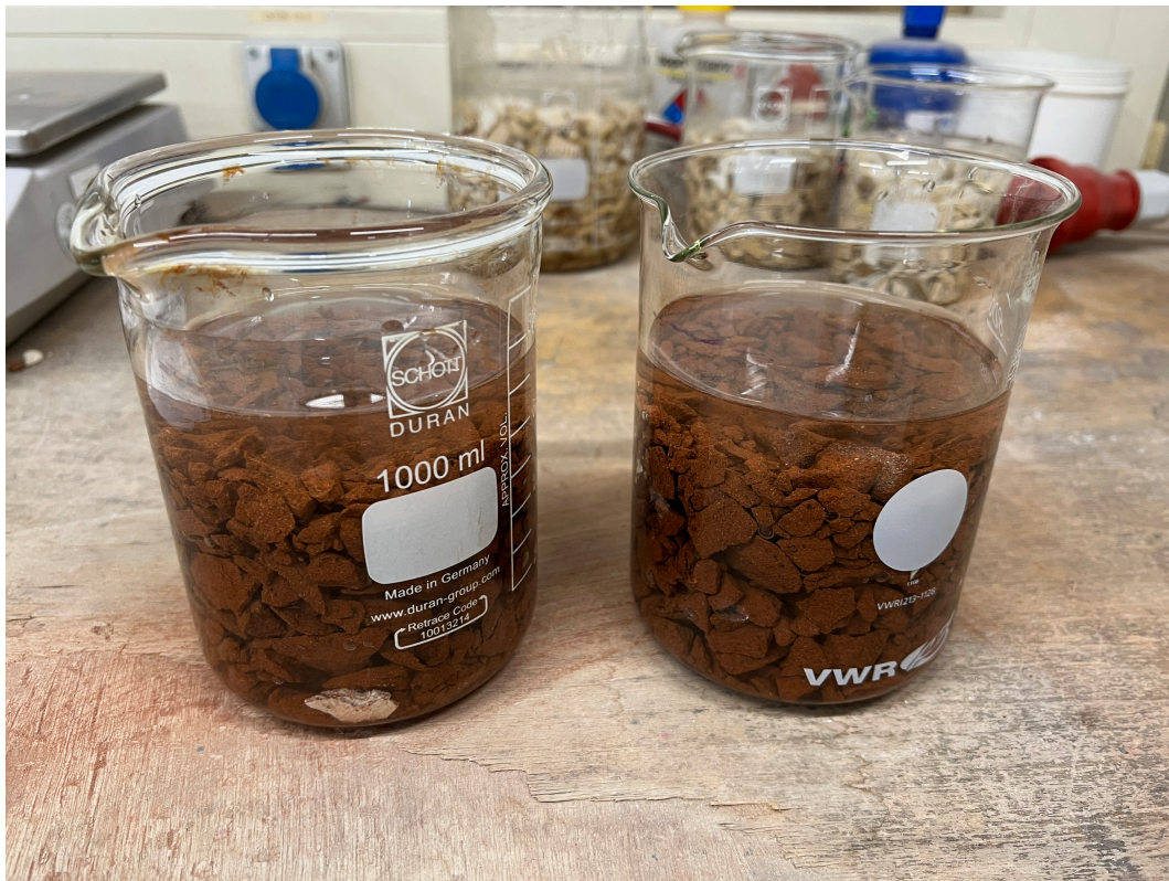
Figure 3.22: Samples are fully submerged in water and kept for 24 hours. In this example, the samples examine the WA of 100% Brick.
