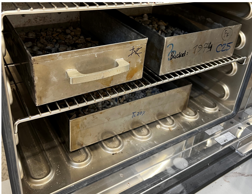
Figure 3.23: Specimens are placed inside an oven at 110°C for 24 hours.
