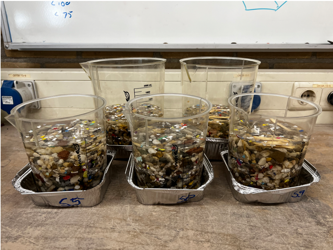
Figure 4.3: Phase 2 samples evaluated for their WA values as part of the standardized procedure
