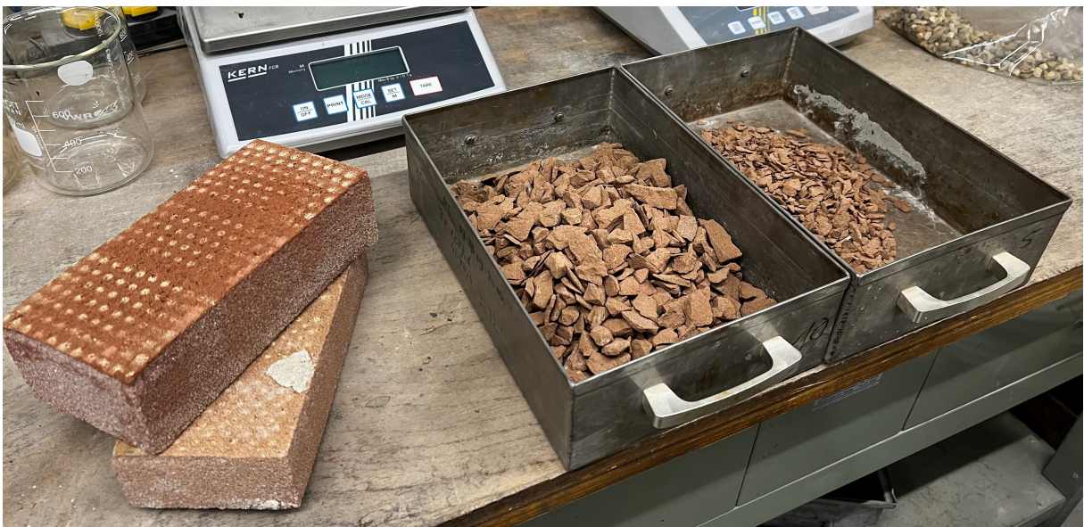
Figure 3.2: Brick transition from whole blocks to 4-16mm particles
