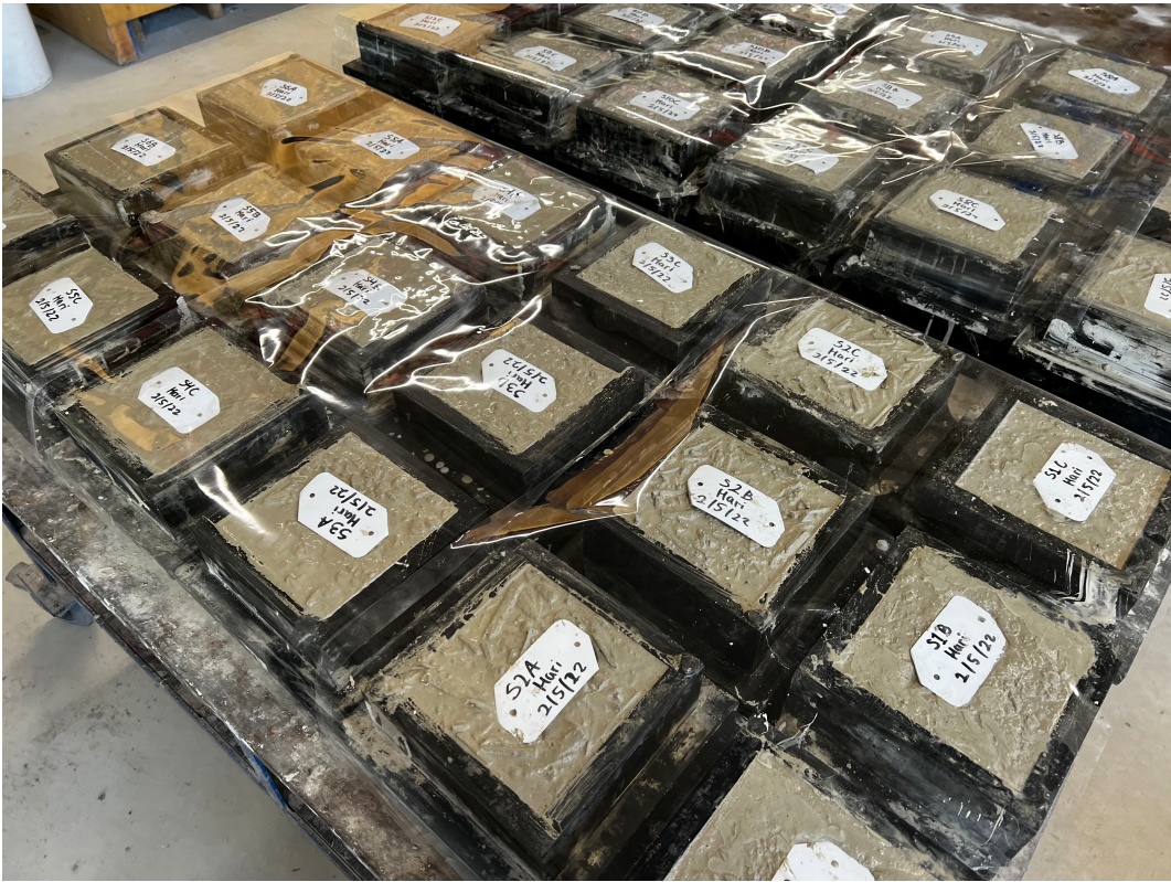
Figure 3.20: Transparent foil is placed on top of the cast specimens to reduce water loss (part of Step 4)
