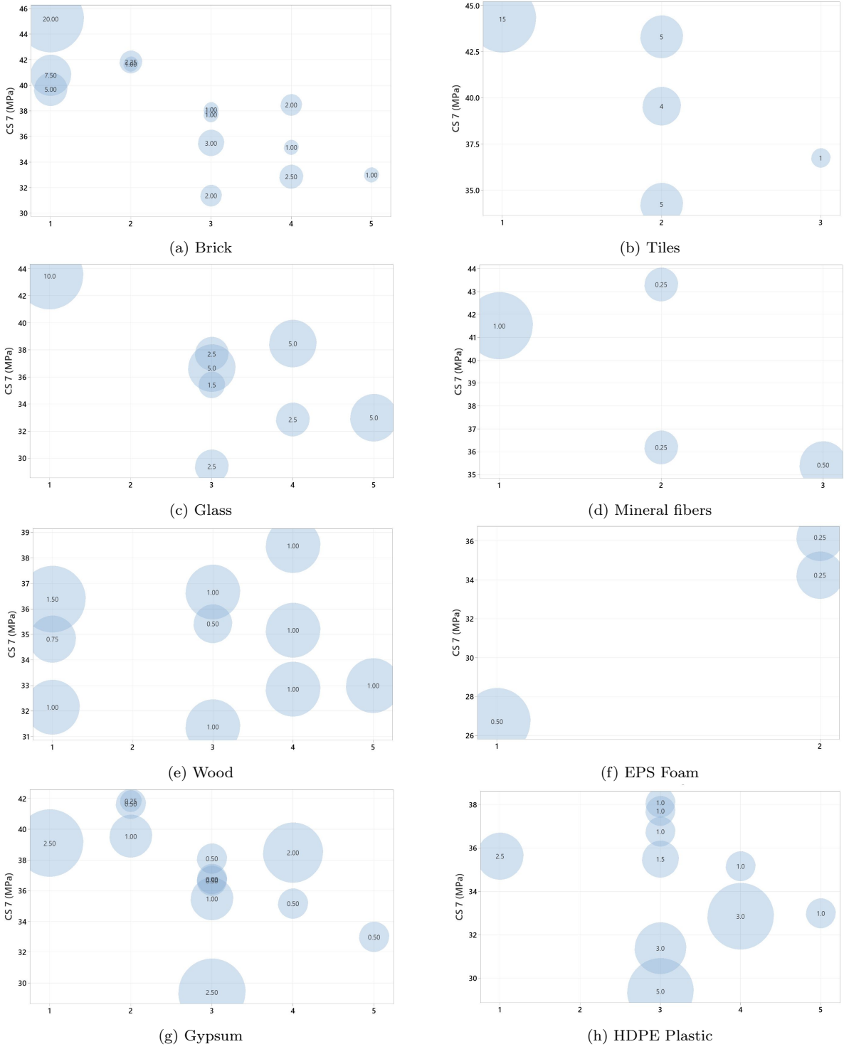
Figure 5.3: Relation between the 7-day strength and the inclusion of a particular contaminant in the recipe alone or in combination with more contaminants
