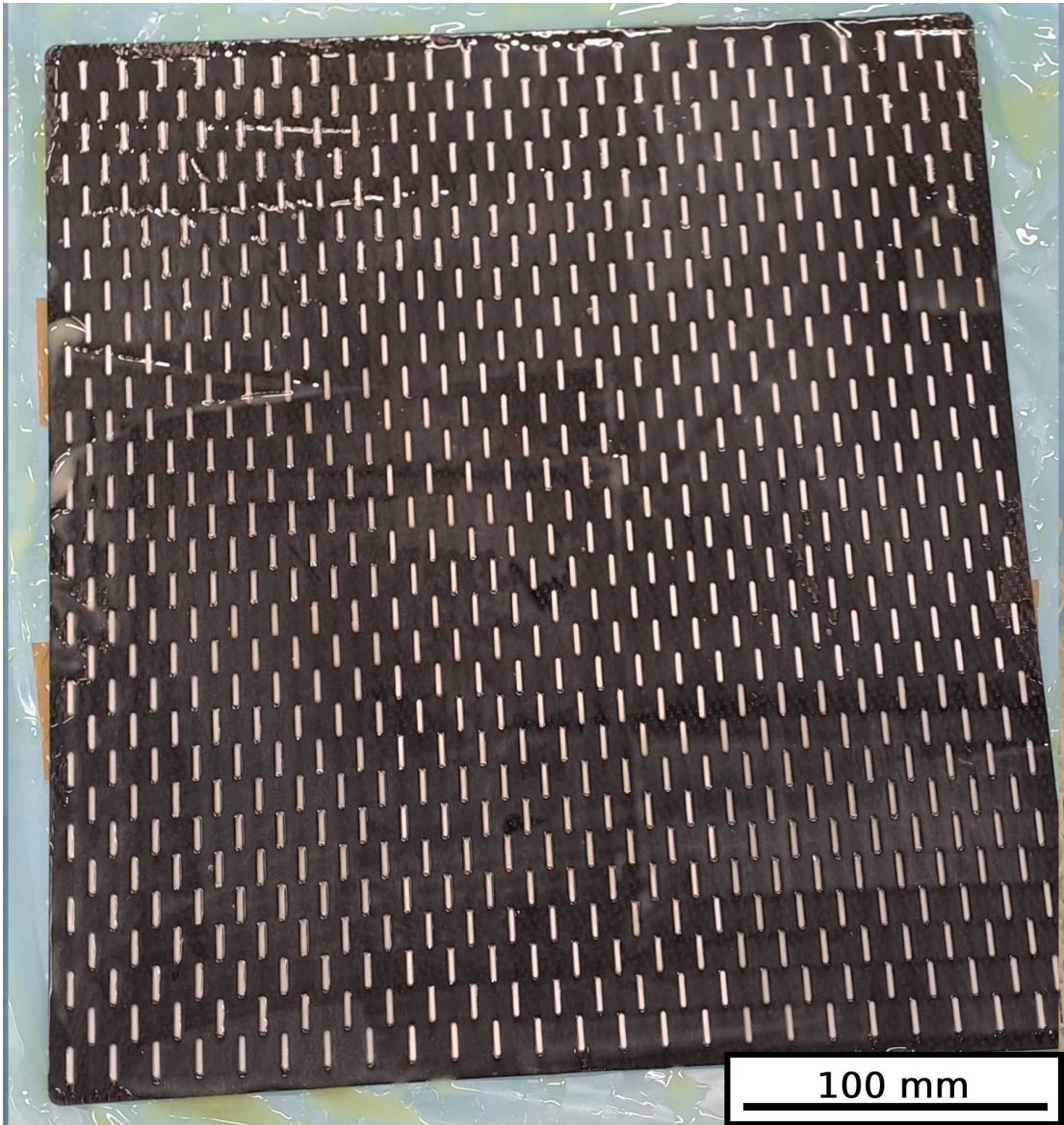
Figure 3.3: Perforated carbon fibre face sheet placed on the jig. The adhesive is applied as if the component was not perforated. Upon removal, the holes remain unobstructed.
