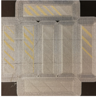
Figure 3.2: Bottom of print created at 20°C and a relative humidity of 70% with print material conditioned at these same conditions 24 hours before printing. The yellow parts in the picture indicate medium print quality.
