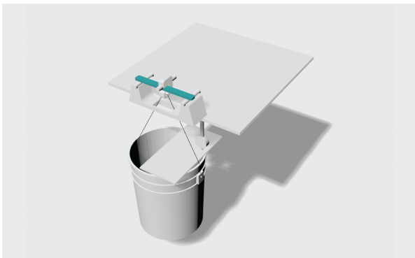
Figure 2.3: A possible bending test using a bucket which can be filled with water to apply force and a gauge to measure elongation
