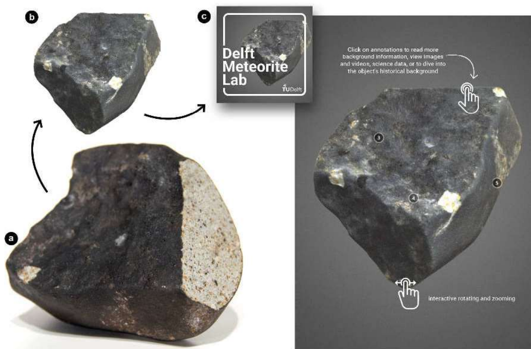
Figure 1 – Overview of the workflow to create a virtual meteorite collection. (a) The Broek in Waterland (L6) meteorite in its current state after imaging and sampling. (b) The digital twin of the meteorite rendered as a 3D model. (c) Hosting in online environment, here Sketchfab.com, to allow users to inspect and rotate the model or access annotations with more information. The collection can be shared and accessed via the convenient short link www.DelftMeteoriteLab.nl .
