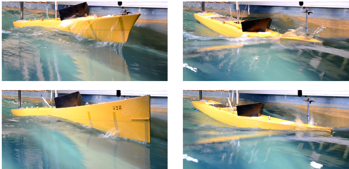
Figure 9: Snapshots of the video recordings of the FSC (upper pictures) and AXE frigate (lower pictures) showing deck wetness in regular waves with a frequency of 0.66 rad/s and a wave amplitude of 2.5 m at a forward speed of 15 knots
