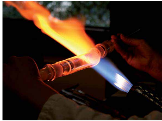
FIG. 5.3 Connection of two tubes in a manual process without lathe
