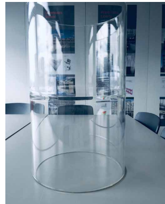
FIG. 5.3 Connection of two tubes in a manual process without lathe
