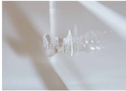
FIG. 6.10 8mm point fitting on 50mm x200 mm flat glass sheet. - The point fitting was chosen as glass in structural architectural applications is commonly connected in a discrete fashion.
