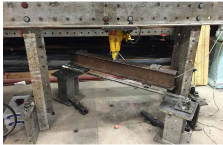
FIG. APP.A.14 Test set-up in 4 point bending jig
