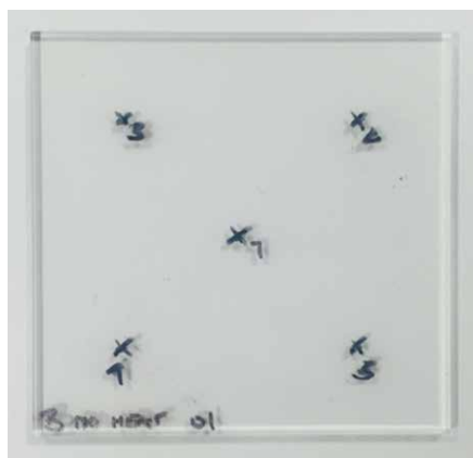
FIG. 5.17 Test specimen with measuring points
