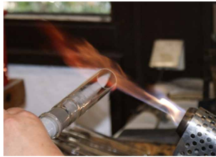
FIG. 6.7 40mm tube attached to 50x200mm flat glass. - Increasing the area of the bond and hence the area that required heating to working temperature, larger tubes were chosen, as it was predicted that these would provide sufficient material stiffness so that load could be introduced into the connection through a shear test.
