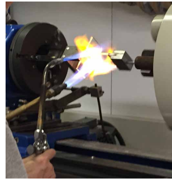
FIG. 6.18 Both flames in use to assure consistent heating of specimen (Flame 1) whilst manufacturing the bond (Flame 2)
