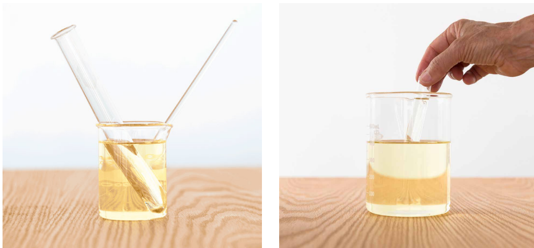
FIG. 5.14 Borosilicate rod and tube submerged in oil
