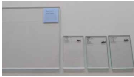
FIG. 2.20 Comparison of glass with varying iron content
