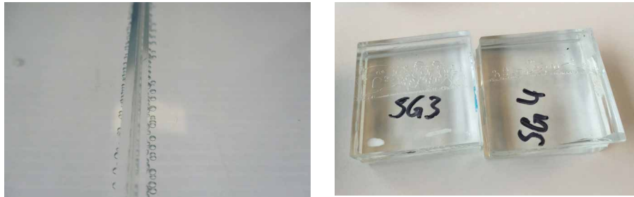
FIG. 7.25 Lamination of SG and TSSA adjacent leading to air bubbles
