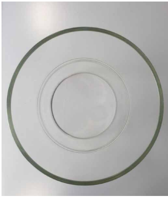
FIG. APP.A.1 Welded glass joint from above
