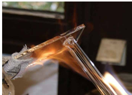
FIG. 6.6 20mm tube (2mm wall thickness) attached to 50 x 200mm flat glass. - Tubular sections are commonly used in scientific glass blowing, so a tube with a small radius and wall thickness was chosen to continue feasibility studies on the manufacturing of the connections.
