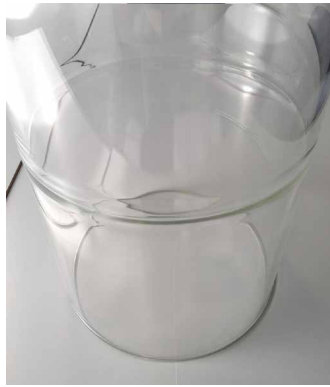
FIG. APP.A.2 Welded glass tube fabricated by Schott
