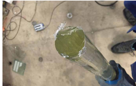
FIG. APP.A.17 Fractured face of glass rod
