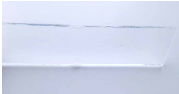
FIG. 7.10 Image heat bonded butt joint
