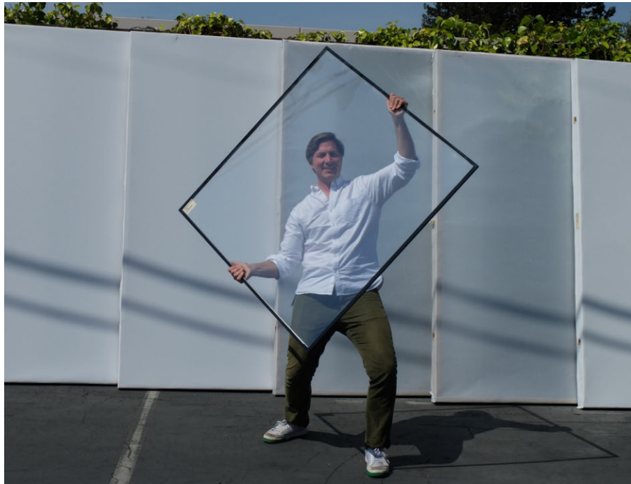
FIG. 7.38 Lightweight IGU made with ultra thin glass laminates (0.7mm+0.7mm/CAV/0.7mm+0.7mm)
