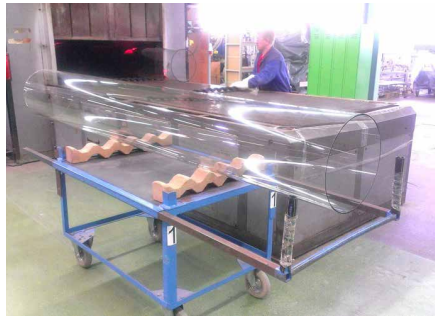
FIG. APP.A.3 3m long extruded borosilicate tube (Schott)
