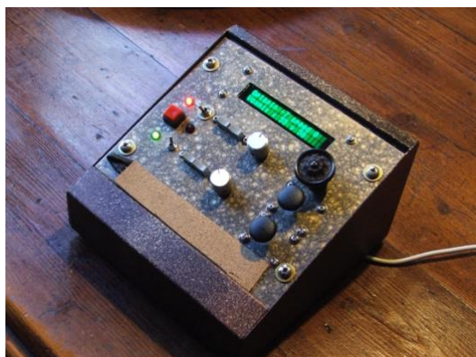
Figure 7 Phidget888 microcontroller physical console interfacing a mixture of dials, joysticks, mode switches and pressure sensor controllers for interactive sonification control.
