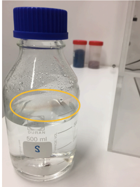
Fig. 3.10. Stain of nanoparticles visible after 1 hour of bubbling with polydisperse particles. At the moment of bubbling, the stain is at water level.
