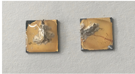
Figure 4.5: Gold contact on the backside of the die
