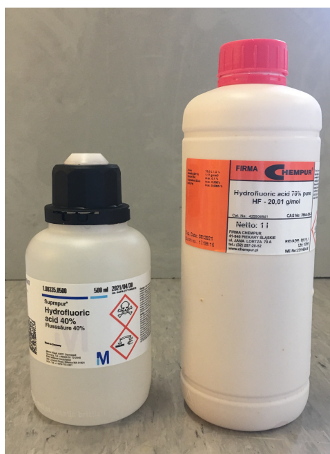
Figure 3.15: HF acid 40 percent and 70 percent used for electrochemical etching process
