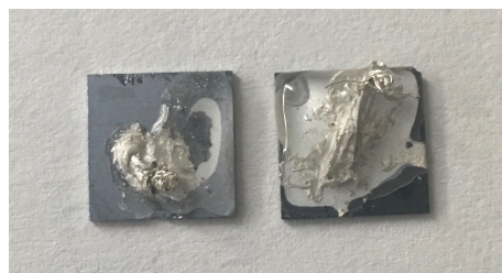
Figure 4.4: Back contact metal Al corrosion
