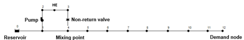
Figure 2. Sanquin full-scale model in EPANET. 0—inlet point/reservoir, 1–4 bypass to the Heat exchanger, HE—heat exchanger, 4—mixing point, 5–11 fictitious points, the mixing point (4), and demand node (12) used to assign measured diurnal flow. The distance between the fictitious points is 500 m, except for the distance between fictitious points 11 and 12, which is 350 m.
