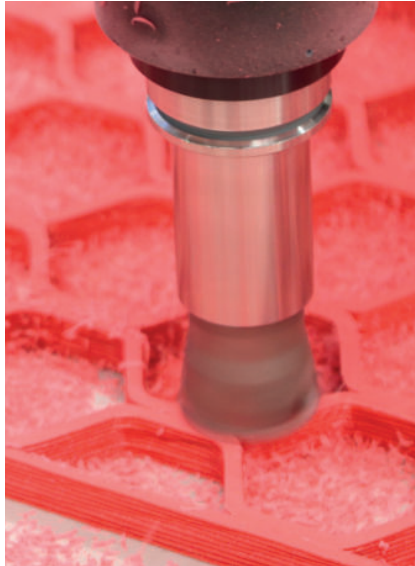
Fig. 7B: Robotic milling of the core surfaces
