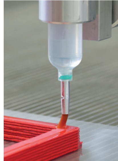
Fig. 7C: Robotic application of the adhesive
