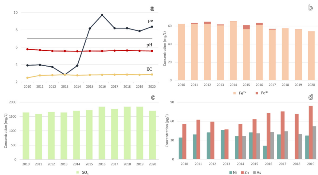
Figure 11. Evolution of groundwater parameters in Schleenhein field: (a) pH, pe (redox corrected and expressed as electron activity) and EC (electro conductivity (mS/cm)); (b) total Fe ( \text{Fe}^{2+} and \text{Fe}^{3+} ); (c) \text{SO}_4 concentrations (mg/L); and (d) trace elements Ni, Zn, and As in ( \mu\text{g/L} ).
