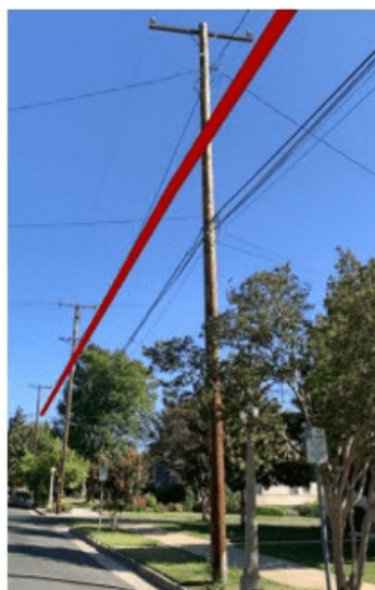
Figure 18. Example of AR scene with the location of a service line superimposed. Here, georeferencing is important to overlay the features on top of the real features. This will be implemented for displaying the derived models on the reclamation site. Taken from ArcGIS Developer: display scenes in Augmented Reality (AR).
