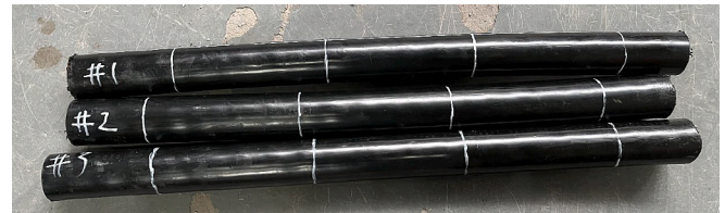
Fig. 16. Cable specimens for bending test.
