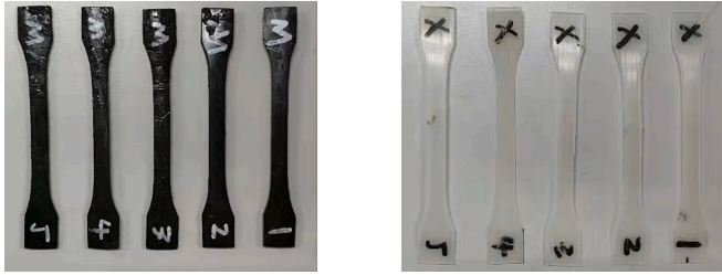
Fig. 11. Dumbbell shape of MDPE (left) & XLPE (right).
