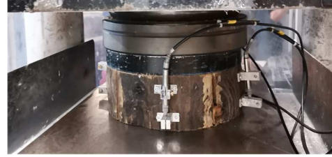
Figure 4. Compression test of a disc sawn from a pile segment.
