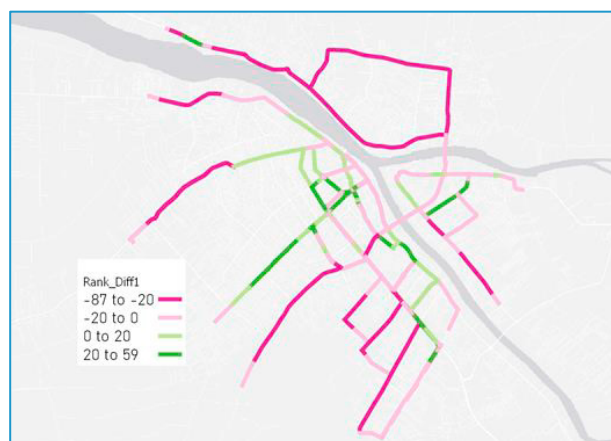
Fig. 6. Difference in criticality rankings between the egalitarian and the utilitarian principles. Negative values imply that the road segment is more critical from the egalitarian perspective (e.g., it ranks 2 nd based on the egalitarian but ranks 8 th in the utilitarian principle), vice versa.
