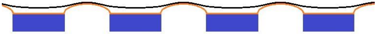
Figure 26. The final design of the tynodes involves bulging membranes to have the desired focusing effect. This would result in a similar issue where the graphene is suspended between the bulges. This would also result in the graphene being washed away during the PMMA removal with acetone.
