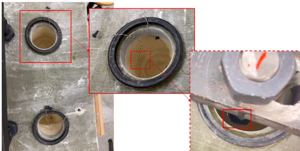
Fig. 7. Location of thermocouples; next to bolt's head (nut) and in foam.
