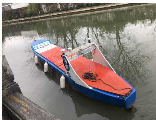
Figure 20: A 7m KVLCC2 model ship.
