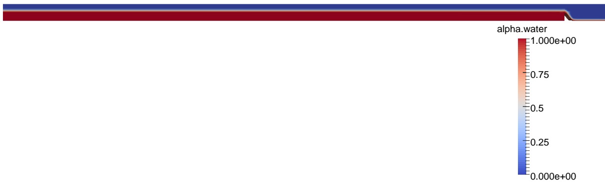
FIGURE 5.1: Initial Simulation of flume without weir but including the control structure. No interface diffusion was observed along the flume.
