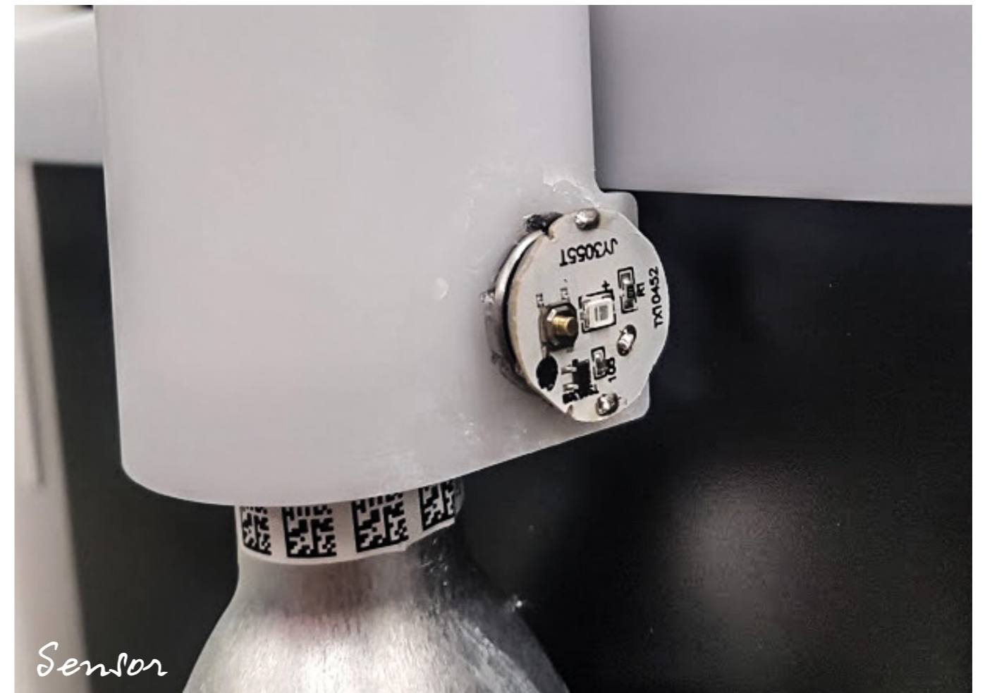
Figure 17. The bicycle light acting as an IoT sensor.
