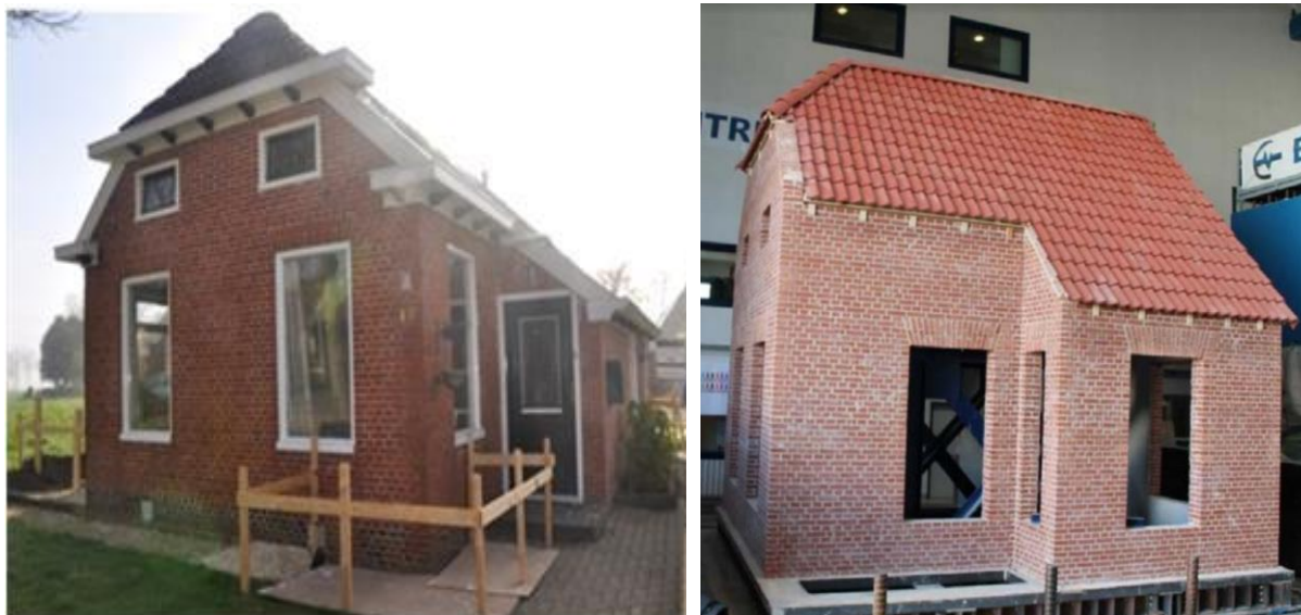
Figure 1: Buildings with construction details similar to those adopted for the shake-table test specimen (from [2]), and actual specimen tested at the laboratory of Eucentre (from [4]).
