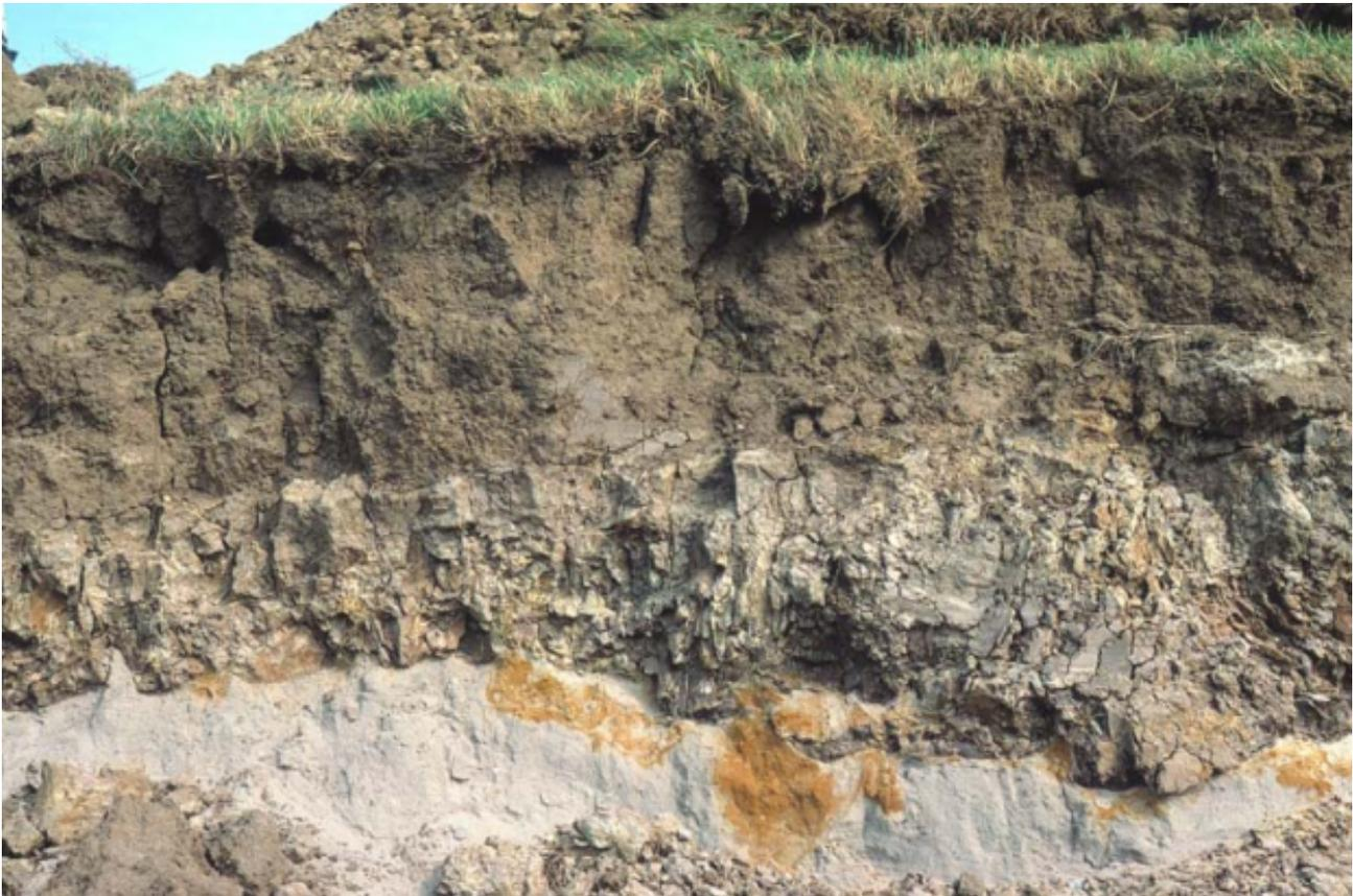
**Figure 1-2:** Soil structure of clay in dikes with the influence of burrowing animals and root penetration. The structure underneath is the result of change in moisture content.
