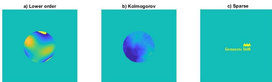
**Figure 2-1:** Example of a) a Lower order, b) Kolmogorov and c) sparse aberrated wavefront.
