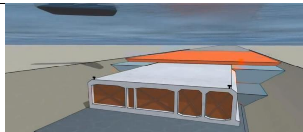
Figure 23: A protective layer (shown in orange) is placed above the tunnel
